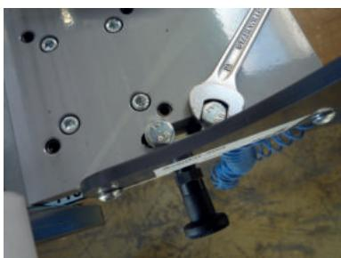
c) Undo latch bolt and screw back in again from the other side
