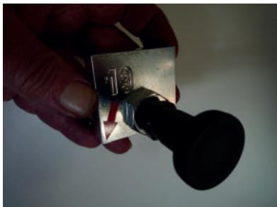
d) Screw fixing screws back in and tighten
